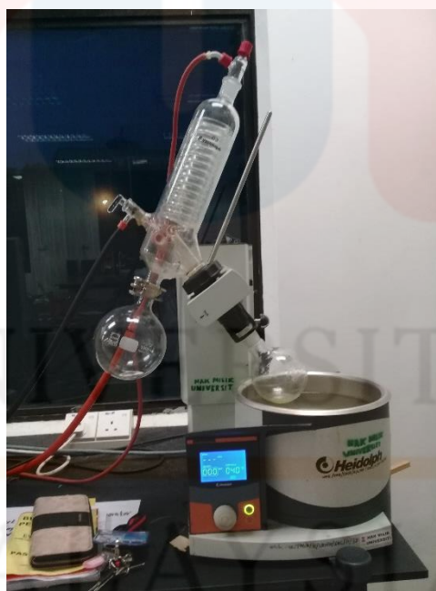
Figure A.5: Filtration and concentration of extracts using rotary evaporator
