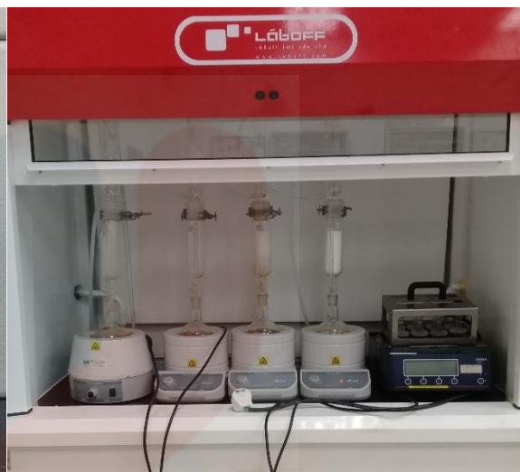
Figure A.4: Solvent extraction using Soxhlet apparatus
