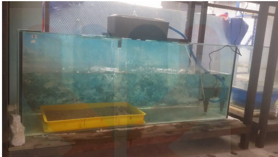
Figure B.7 Closed-culture experimental tank system for Asian Clam culturing.
