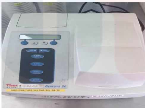
Figure 3.5: Spectrophotometer Thermo Scientific Gynesis 20
