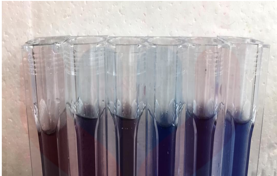
Figure 3.6: Dilution factor of 500X, 200X, 100X, 50X, 20X, and 10X in Bradford reagent
