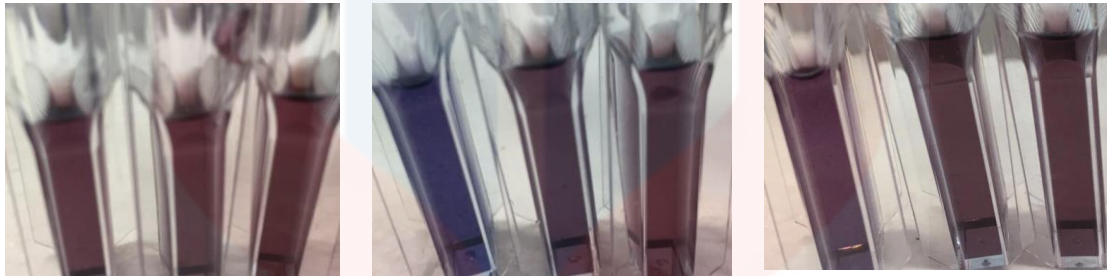
Figure B.1: Bradford assay of protein sample with buffer PBS, RIPA, and RIPA + Pi and ratio 1:1, 1:3 and 1:5 (from left)
