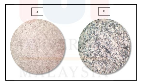
**Figure 4.14:** Thin section of limestone under plain polarize light (PPL) on the and cross polarize light (XPL) on the (b). Both of thin section is under 4x10 magnification.
