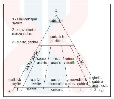
Figure 4.18: QAPF diagram used for granite classification
