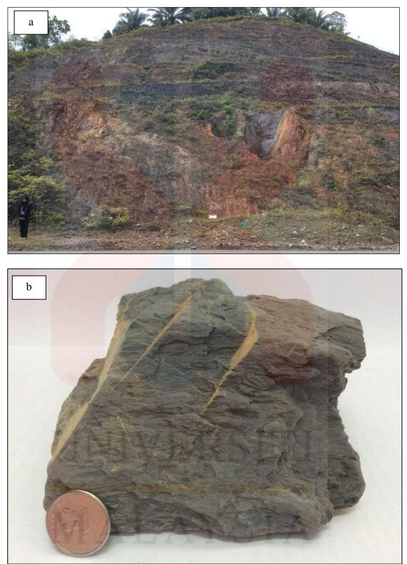
Figure 4.10: (a) The field observation of slate outcrop along Jalan Jelawang- Gua Musang. (b) The hand specimen of the slate.
