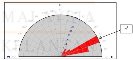
Figure 4.22: Joint analysis on granite by using GeoRose Diagram
