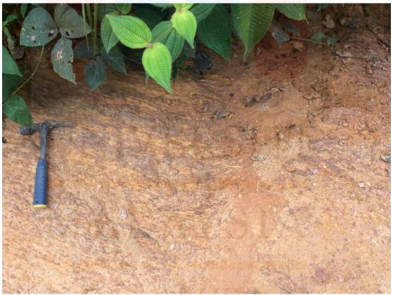
Figure 4.23: Minor fold occurred at mica schist outcrop.
