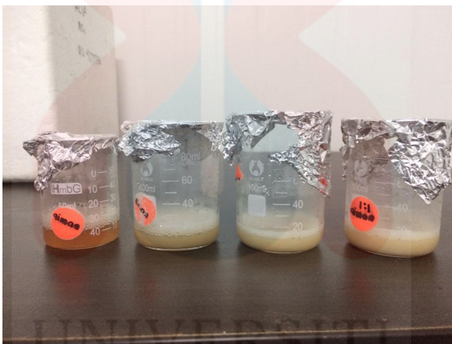
Figure 3.1: The solution after incubating for 2 hours at 4°C with different concentration of AS, 0%-20%, 0%-40%, 0%-60%, 0%-80% (from left to right)
