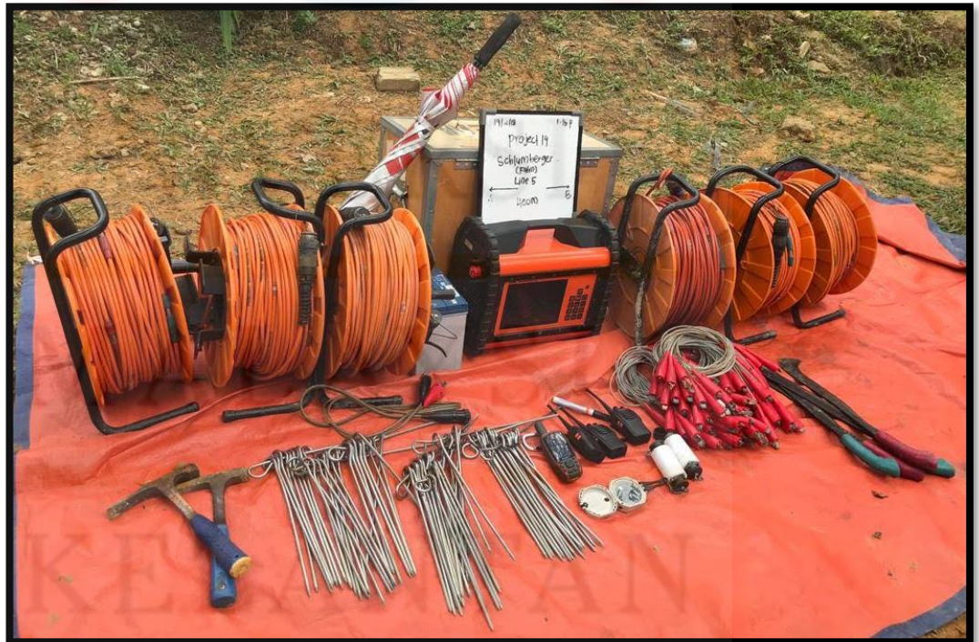
Figure 5.1: Equipment for electrical resistivity investigation
