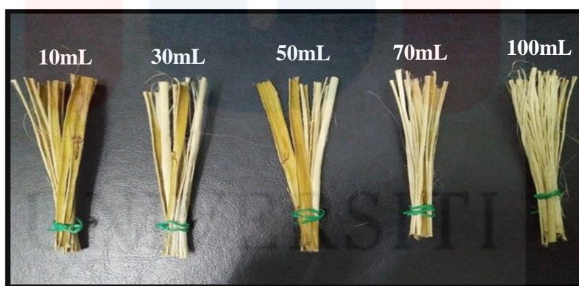
Figure 4.2: Kenaf bast fiber from enzyme combination of 100 % pectinase for 24 hours
