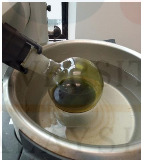
Figure 2: L.zeylanica methanolic leaves using rotary evaporator
