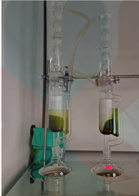
Figure 1: L.zeylanica methanolic leaves using soxhlet extractor
