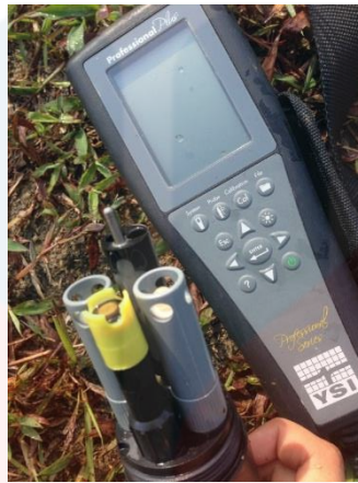
Figure 1 : Water multi-parameter used to measure water quality
