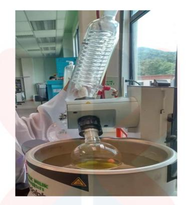
Figure 5.3 : Removing solvent using Rotary evaporator
