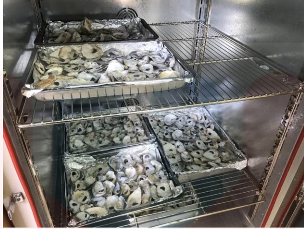
Figure A3: Washed oyster shell were placed in oven for drying process.
