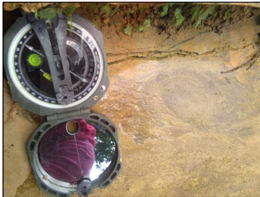
Figure 4.23: Spheroidal weathering that has circular shape with look like peel onion. Picture were taken with azimuth N 40 0 W at station 14 .
