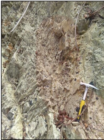
Figure 4.21: Jointing on rhyolite rock that cause physical weathering. Picture were taken with azimuth S 15 0 W at station 6 .
