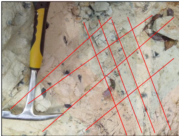
Figure 4.60: The cross joint structure on rhyolite rock. The picture was taken at station 5.
