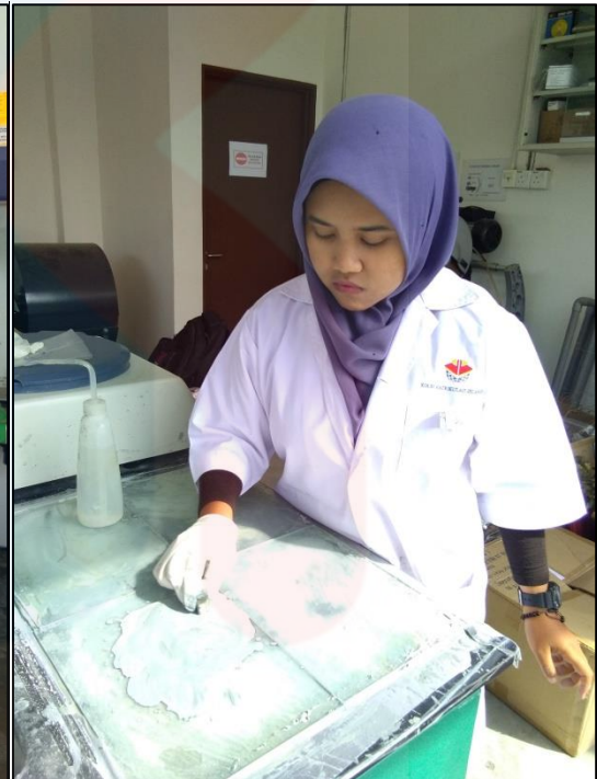
Figure 3.3: Polish the surface of cutting rock.
