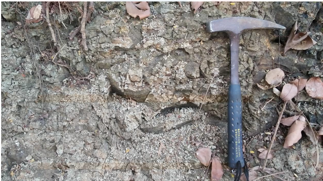
Figure 4.4 Claystone outcrop that already undergone weathering process. Weathering process that involve are physical, chemical and biological.
