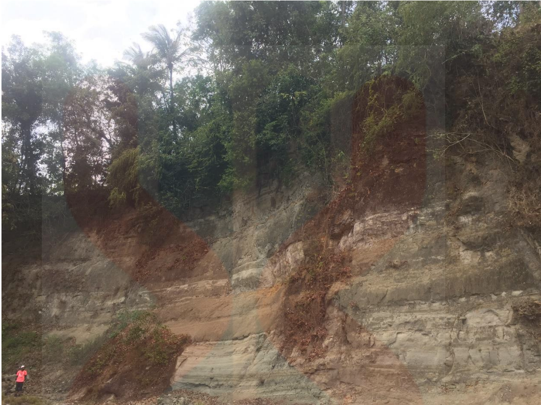
Figure 5.22 Thick bed of claystone and sandstone, which is interlayering to each other.
