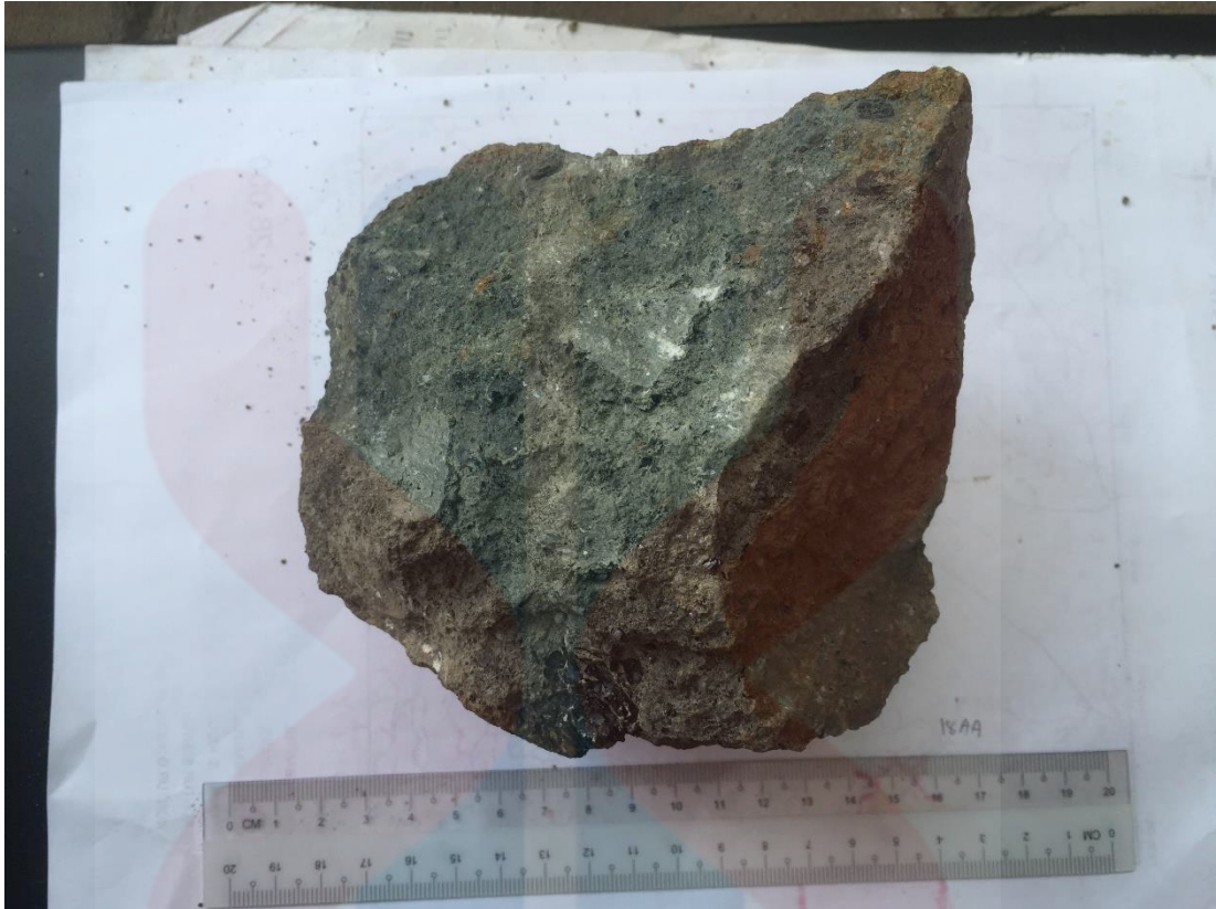
Figure 4.7 Andesite hand specimen. At the below part of sample, seen a hornblende mineral.
