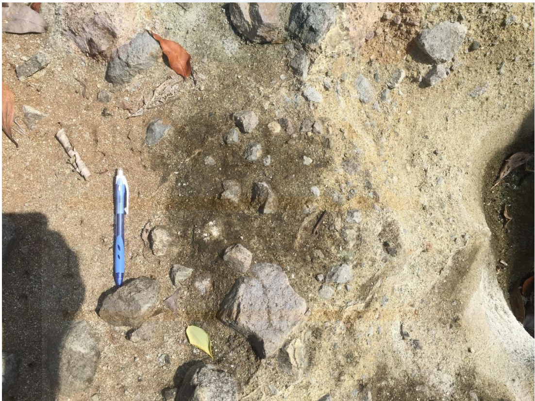
Figure 5.14 Breccia, matrix-supported. The matrix are sandstone and the fragment are andersite material from Nglangeran formation.
