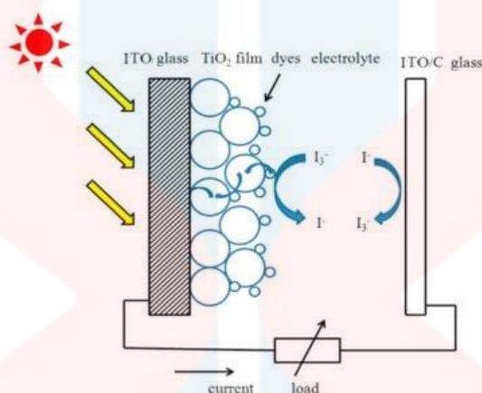
Figure 2.3: The mechanism in DSSC (Ranabhat *et al.*, 2016).
