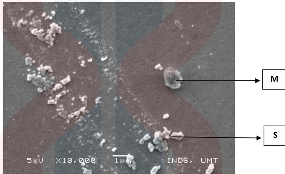
Figure 4.5: SEM image of the mixed dye 30**M**: 1**S** on ITO glass.
