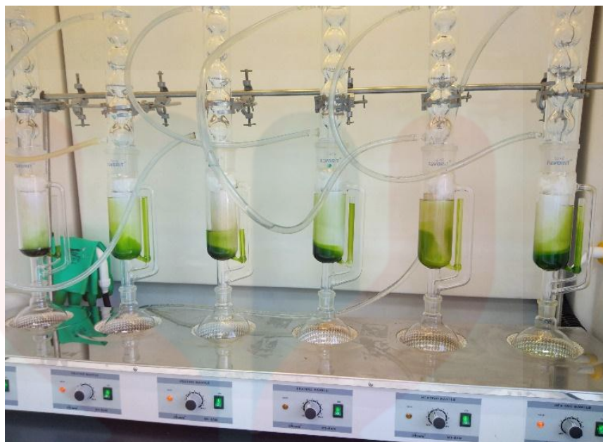
Figure 3.2 Soxhlet extraction setup
