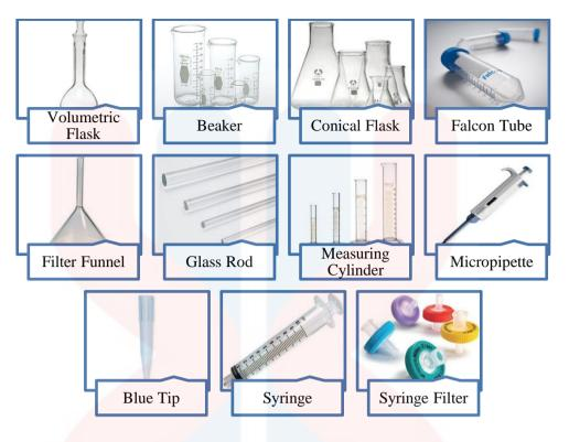
Figure 3.5: Apparatus for sample digestion.
