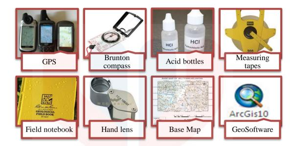
Figure 3.2: The tools and stationaries used for geological mapping.
