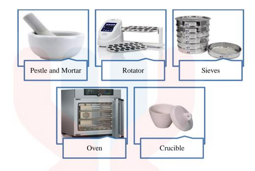
Figure 3.3: Tools for sample pulverization.
