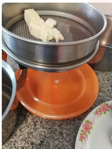
Figure 2.1: Experiment of conducting dripping time test on control ice cream.
