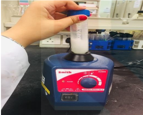
Figure 5.1: Scrubbing process using vortex
