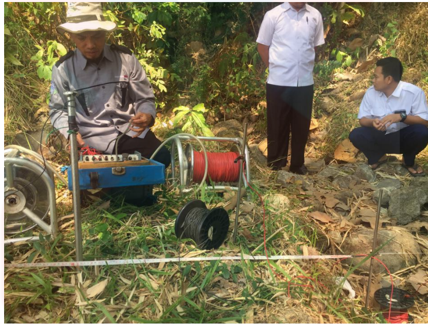
Figure 5.2: Electrode configuration for 1-D Schlumberger array for VES.
