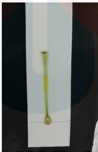
Figure 4.1 Silica gel TLC plate with separated compounds from Christia vespertilionis leaves extract
