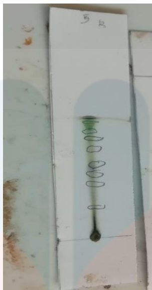
Figure 4.2 Silica gel TLC plate with separated compounds from Christia vespertilionis has been outlined and heated. The present of coloured spot was not detected
