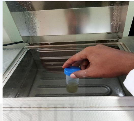
Figure B.6: using hot water bath to melt the fat in liquid form at 70°C.
