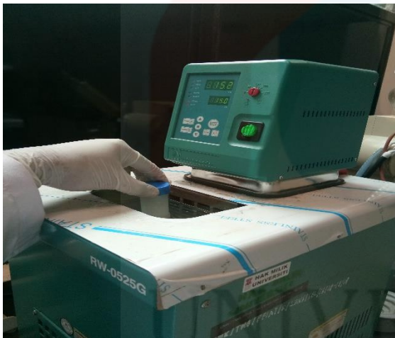
Figure B.5 : Using cold Water Bath to study the effect of Difference cold temperature
