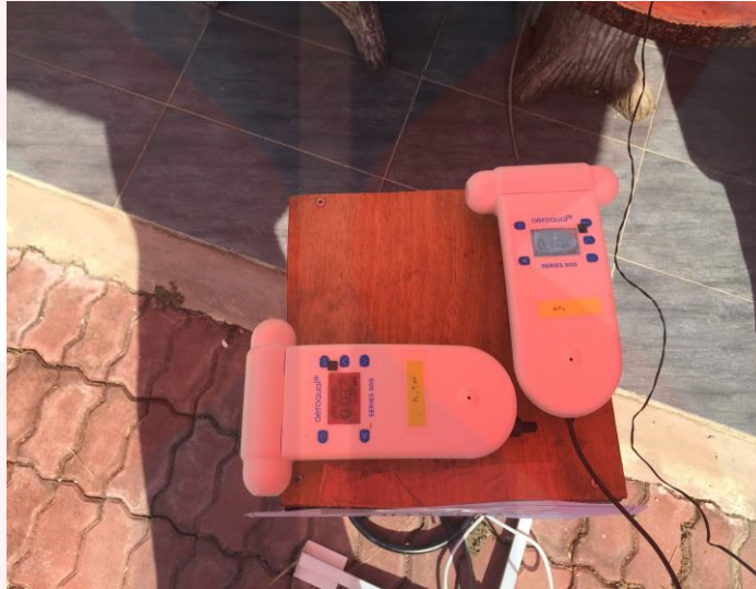
Figure A1: Aeroqual series 500 (ozone and nitrogen dioxide sensor) set up in monitoring site under a canopy umbrella
