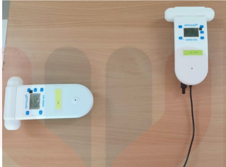
Appendix C: The position of both aeroqual with O 3 and NO 2 sensors
