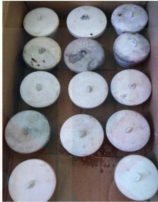
**Figure 3.10:** Soil Samples and Crucibles After the Combustion Process.
