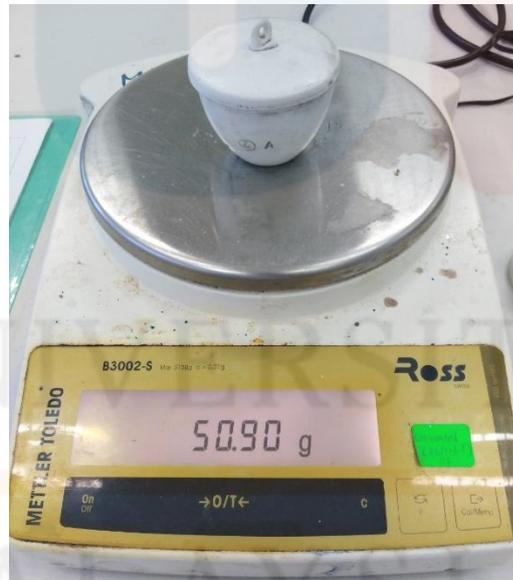
**Figure 3.7:** Soil Sample and Crucible Weighed Using Electronic Balance Instrument.
