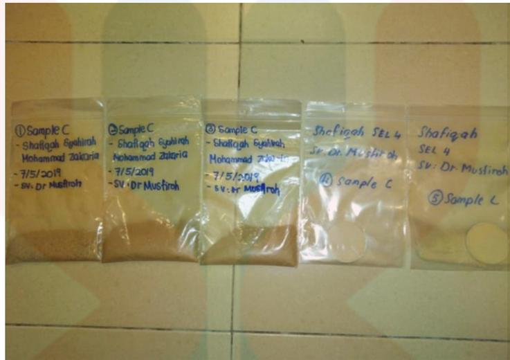
**Figure 3.11:** Soil Samples for X-Ray Fluorescence (XRF) Analysis.
