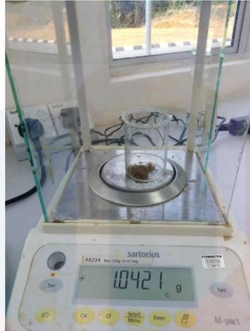
**Figure 3.15:** Soil Sample Weighed in Beaker Using Analytical Balance Instrument.
