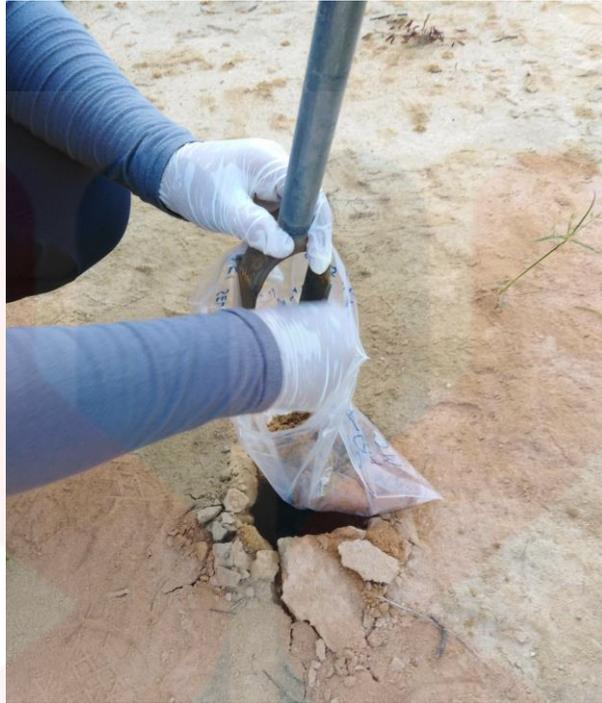
**Figure 3.5:** The Process of Collecting the Soil Sample at Sampling Site.
