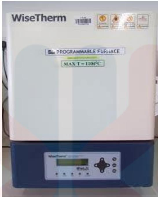
**Figure 3.8:** Muffle Furnace Instrument Used in Organic Matter Analysis.
