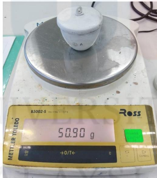
Figure 3.7: Soil Sample and Crucible Weighed Using Electronic Balance Instrument.
