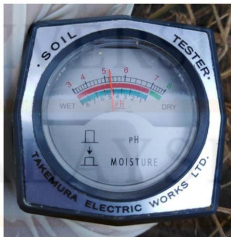
**Figure 3.6:** Soil pH and Moisture Meter Used in In-Situ Analysis of pH and Moisture Content of the Soil.
