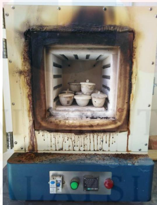
**Figure 3.9:** Soil Samples and Crucibles Placed in Muffle Furnace for Combustion Process.
