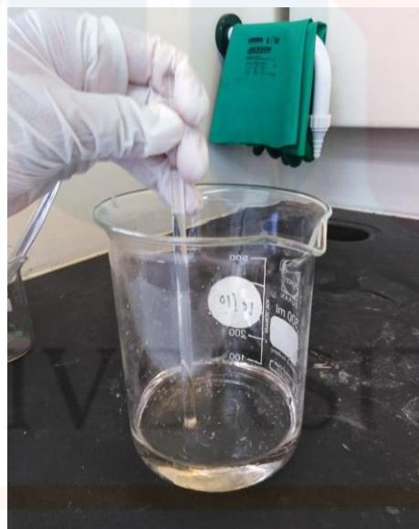
**Figure 3.14:** Preparation of 5% Chromotropic Acid Solution.
