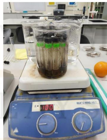
**Figure 3.17:** Warmed-Over the Mixture of Soil Samples, 96% Concentrated Sulphuric Acid Solution and 5% Chromotropic Acid Solution Boiling Water Bath For 1 Hour At 100°C Using Hot Plate Instrument.
