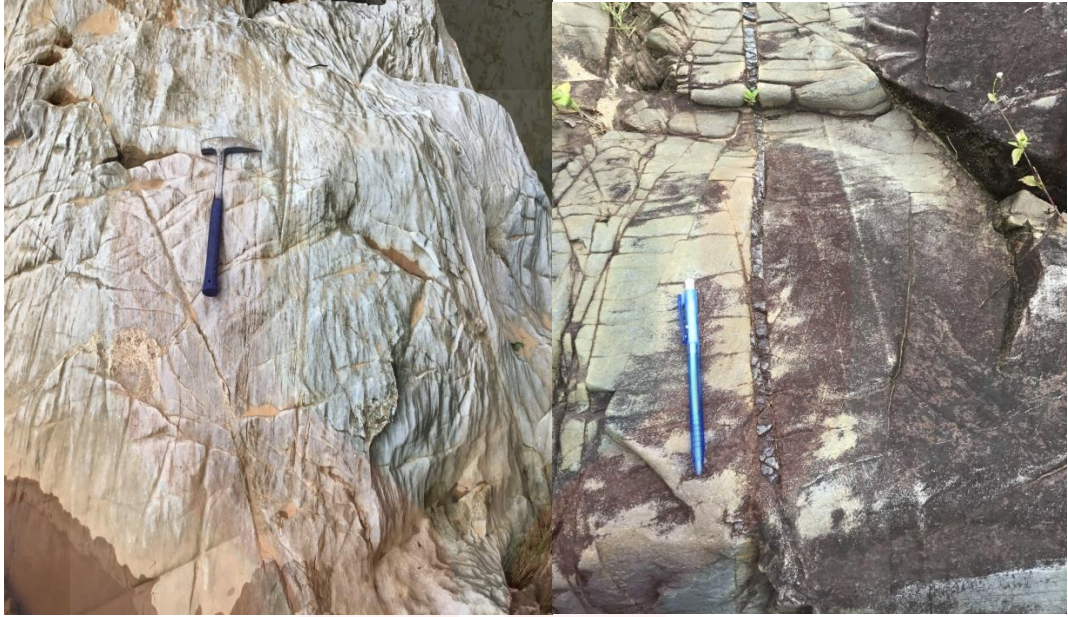
Figure 4.42: Shear joint at Marble. Coordinate: N 05° 46' 20'', E 101° 44' 55.8'' (left). Extension Joint. Coordinate: N 05°46' 35.3'' E 101° 44' 51.7'' (right).
