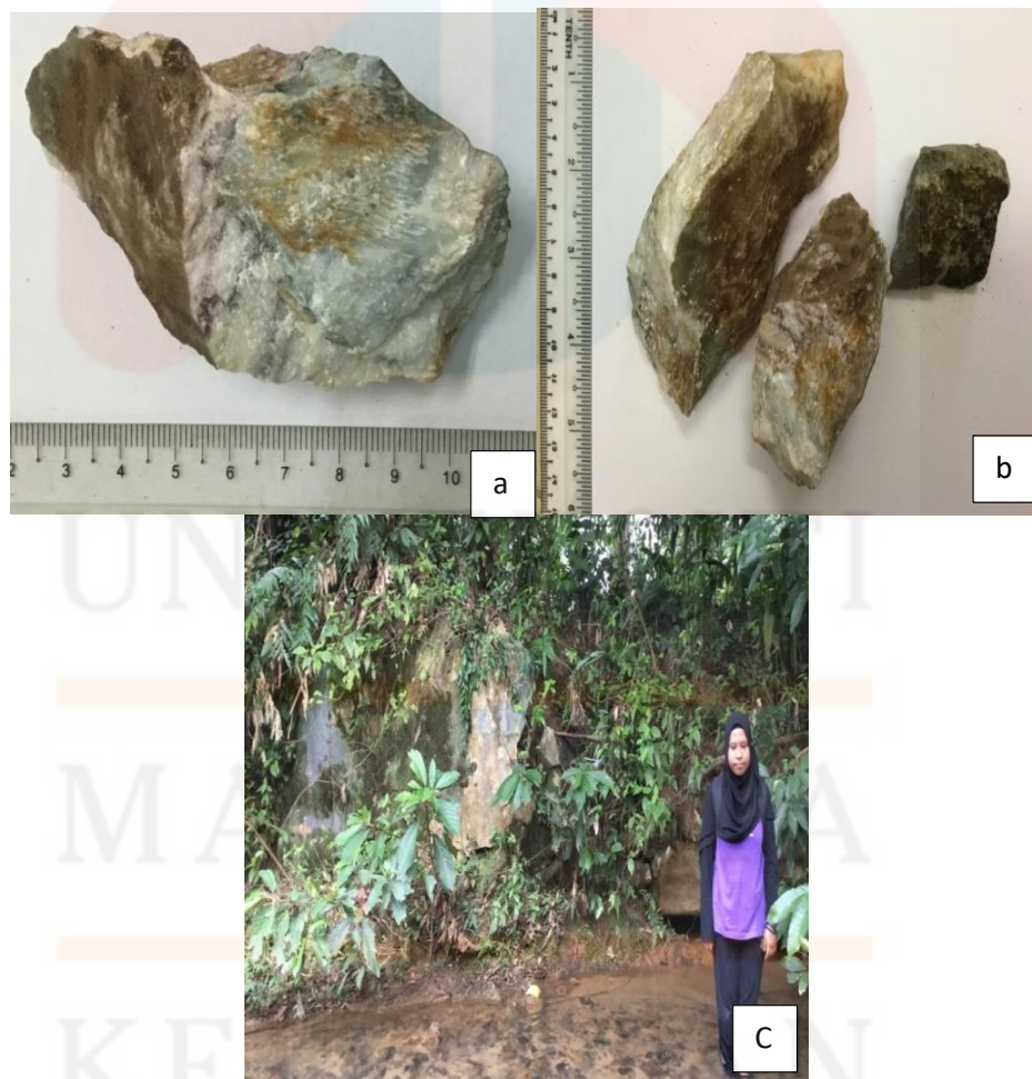
Figure 5.11: The lithobiontic coatings on marble. (a) Closer-focused on lithobiontic coating at marble. (b) The marble hand specimen which coated with lithobiontic coating. (c) The outcrop of marble which covers by biological weathering and coated by lithobiontic coatings.
