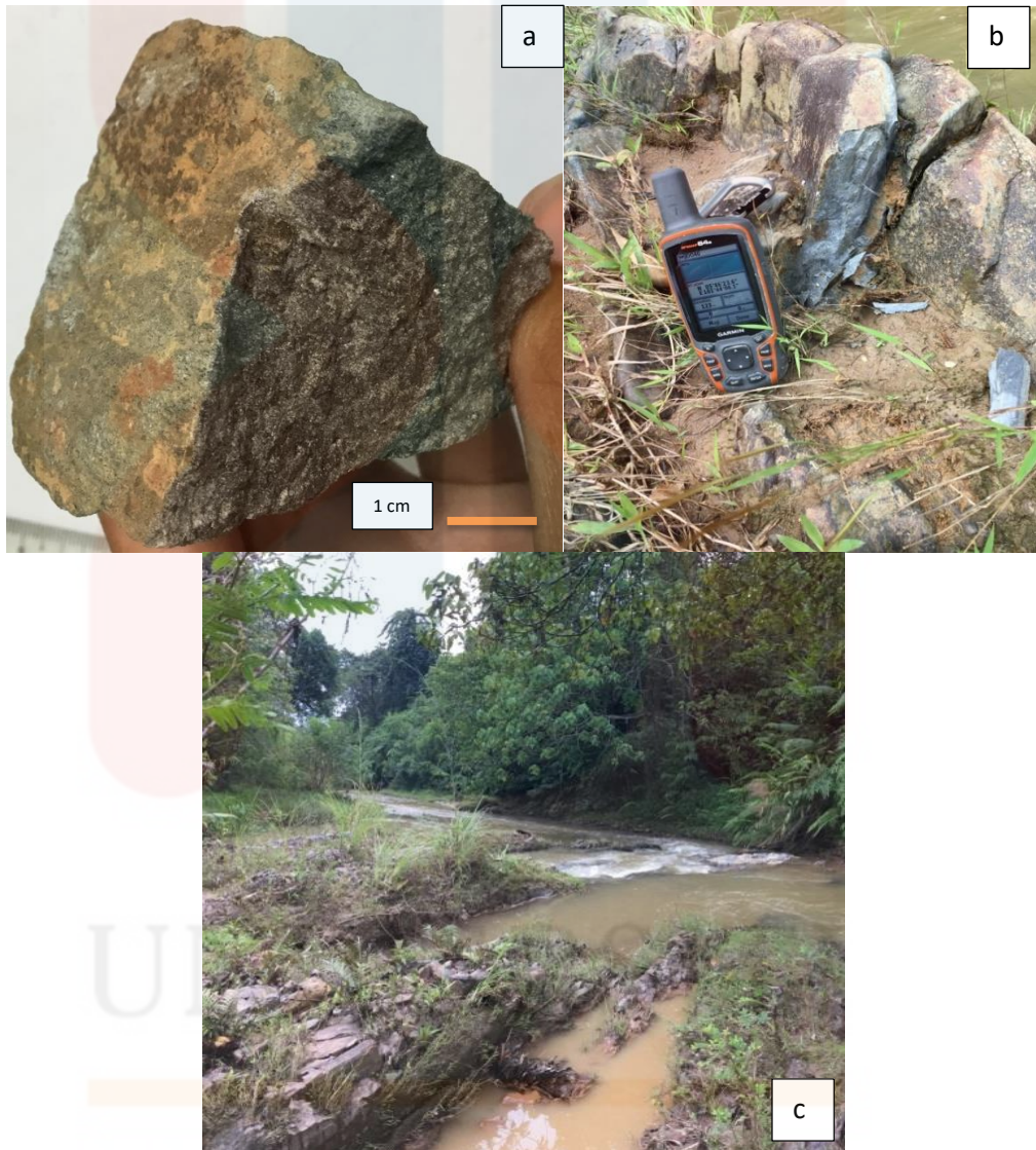
Figure 5.10: The dust film of Schist rock. (a) Hand specimen of schist that covers with dust film. (b) Schist that coated with dust film. (c) The outcrop of schist that located at Sg.Tadoh.
