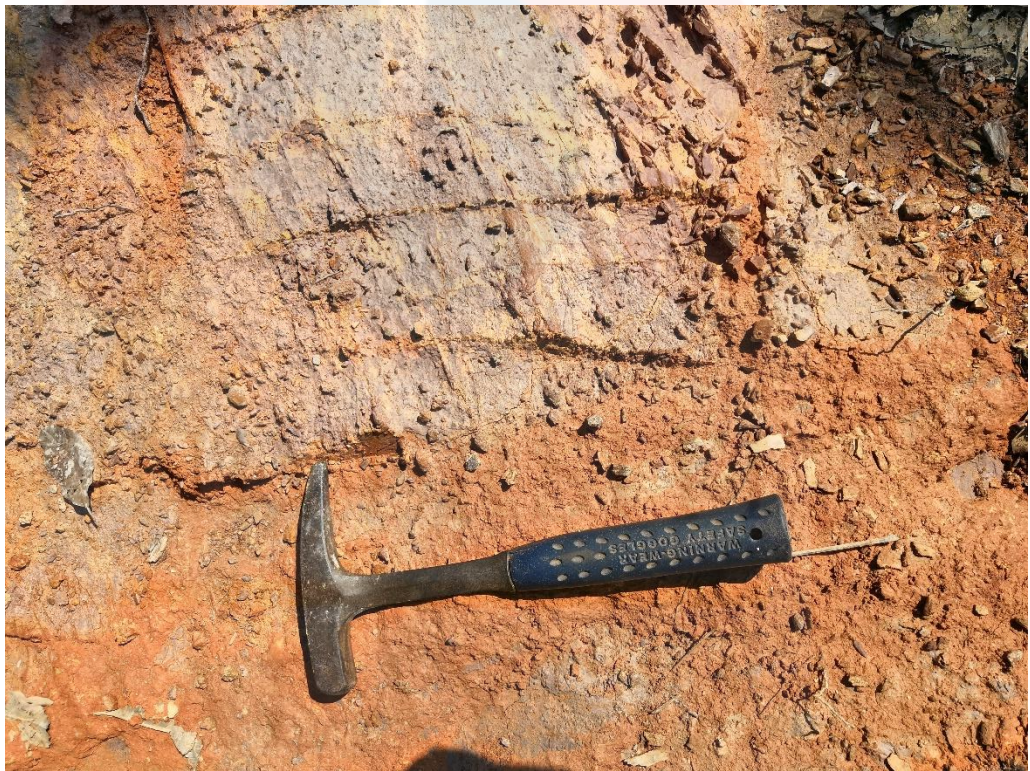
Figure 4.30 : The shear joint
