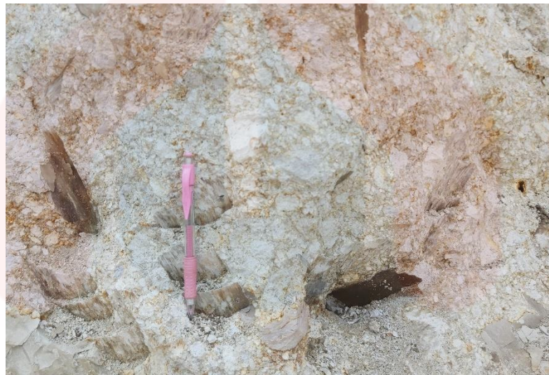
Figure 4.26: Pumice structure found in Breccia Tuff.
