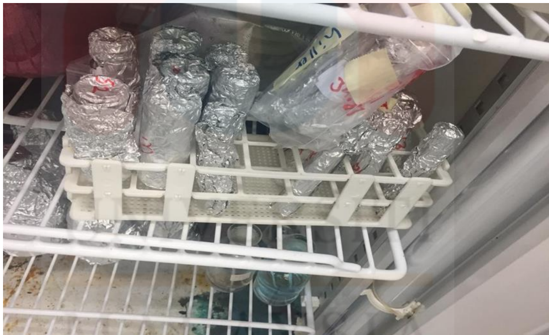
Figure B4: The samples need to wrapped with baked aluminium foils and stored in chiller.
