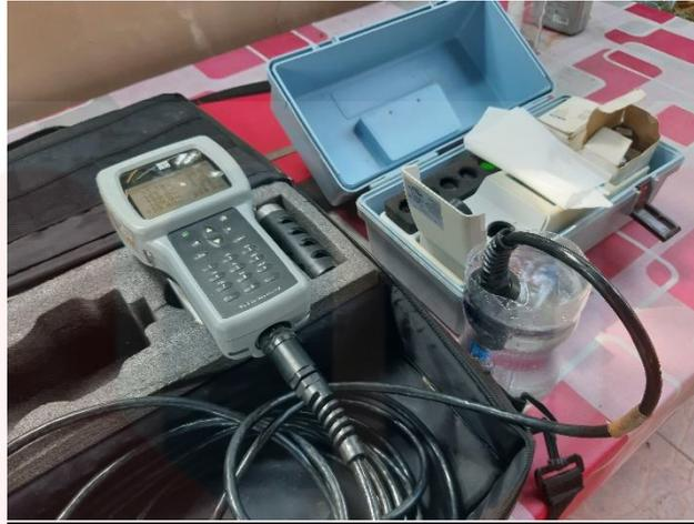
**Figure 3:** In situ geochemical analysis of water sample using YSI Multiparameter
