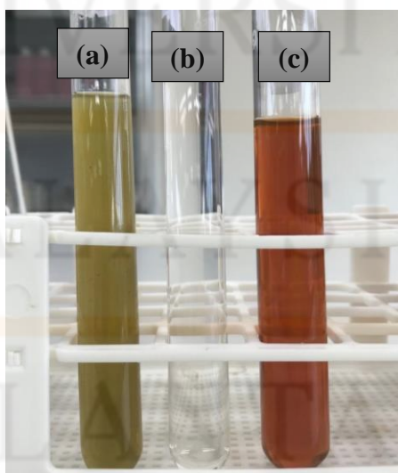
Figure 4.1: Three test tube containing A. microphylla extract (a), \text{AgNO}_3 solution (b) and AZO-AgNPs (c)
