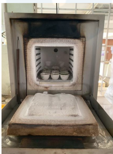
Figure 3.1.5 (b): Crucibles are labelled and kept in the muffle furnace at 600 0 C for 2 hours
