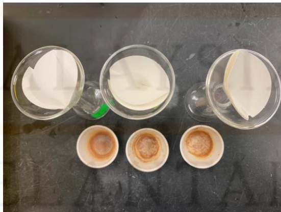
Figure 3.1.6 (b): Sample after the ashing method
