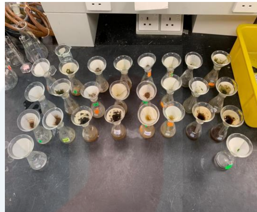
Figure B.8 Collection of residues of samples for HPLC analysis
