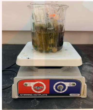
Figure 3.1.2 (d): Samples were heated for 18 minutes on stirring hot plate
