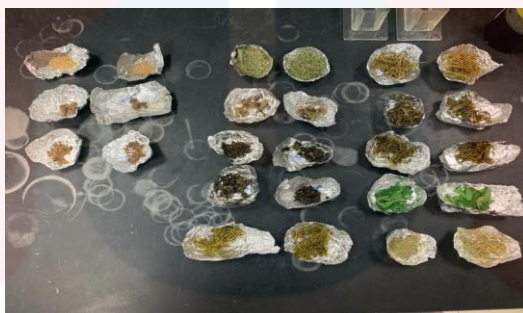
Figure 3.1.2 (a): 0.5g of each sample is weighed and placed on aluminum foil
