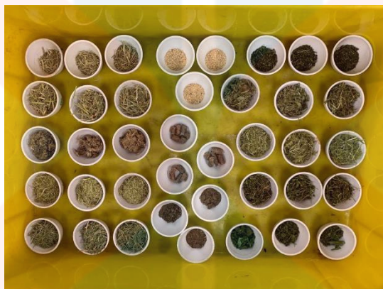
Figure 3.1.5 (a): 2g of dried sample were mixed, weighed and then kept in the crucible
