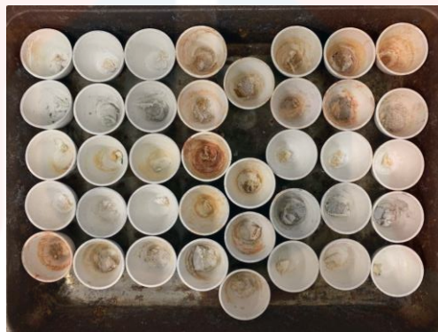
Figure 3.1.6 (b): Washing of dried silica for almost three to four times
