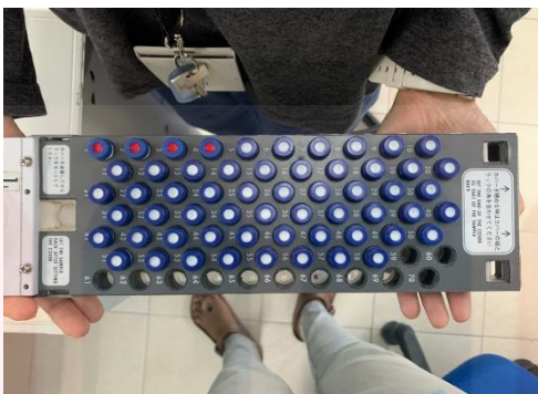
Figure 3.1.4(a): Oxalate extraction in the vial tray ready for HPLC analysis
