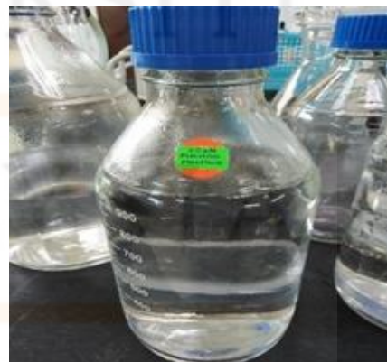
Figure B.6: 20mM of potassium phosphate as eluent a for HPLC analysis
