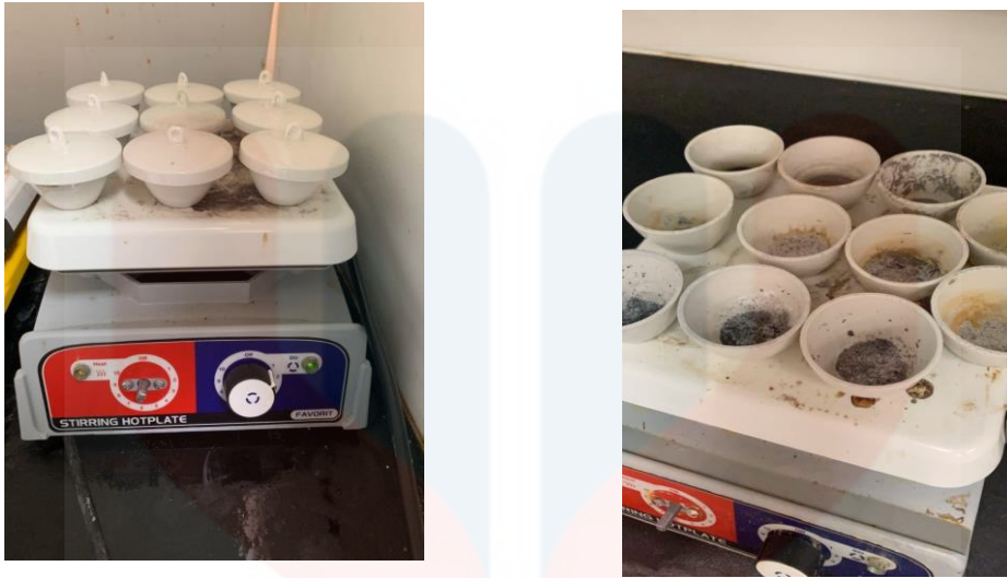
Figure 3.1.6 (a): Dehydration process after HCl were added to the remained ash
