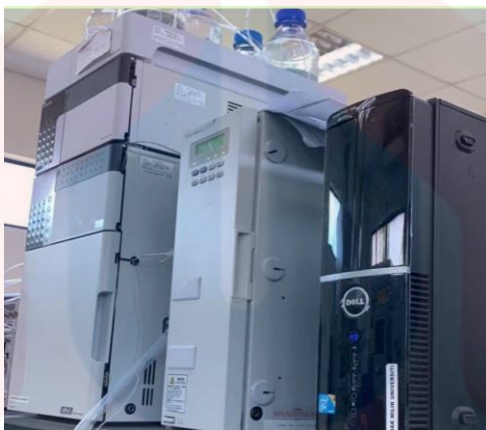
Figure 3.1.4(b): The HPLC machine
