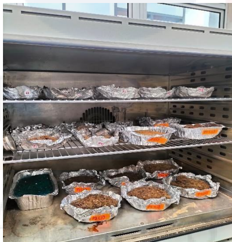
Figure 3.4: The process of drying the soil using laboratory oven
