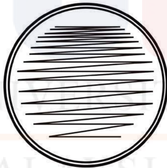
Figure 3.1: The continuous streak method for microorganisms culture
