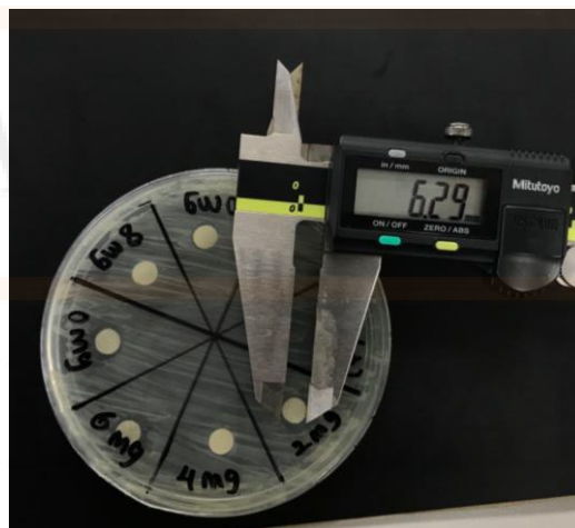
Figure 3.4: The measurement of the diameter inhibitory zone by digital vernier calliper
