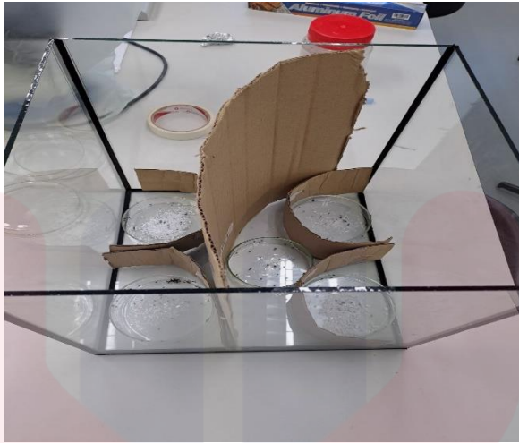
Figure 3.2 Preparation before placing rice beetles in five types of plastic in an aquarium
