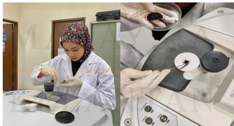
Figure 3.9 Use FTIR to evaluate the presence and composition of microplastics.
