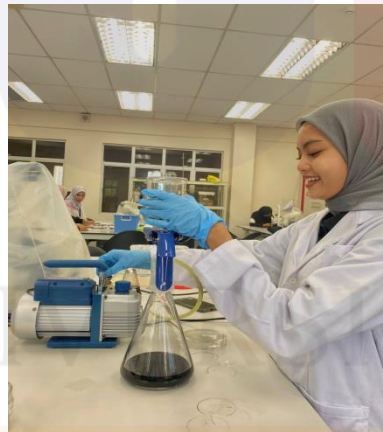
Figure 3.5 Use a vacuum filtration system for the samples that have been shaken.
