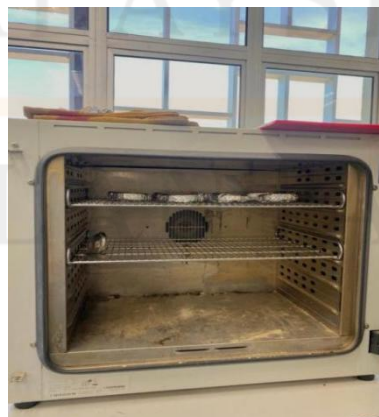
Figure 3.6 Filter papers in the petri dish and put it in the oven ( 47^{\circ}\text{C} ) for 2 hours.
