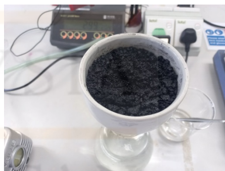
Figure C6: Activated carbon was washed to achieve pH 7
