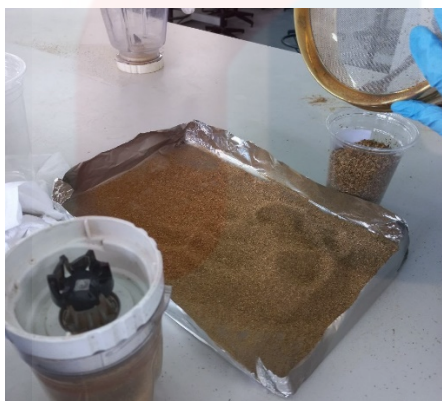
Figure C3: Dried pineapple peel was ground and sieve 500 \mu\text{m}
