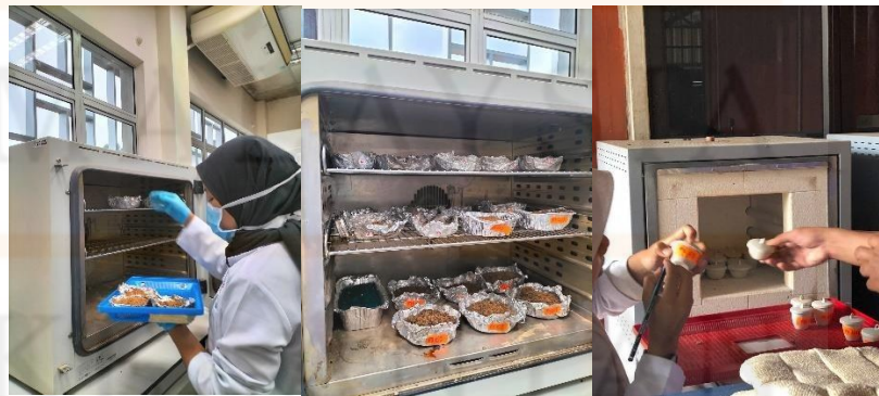
Soil sample being weight, placed din crucible cup, baked in oven to dry the soil and put in furnace to turn the soil into ash and measure OM
