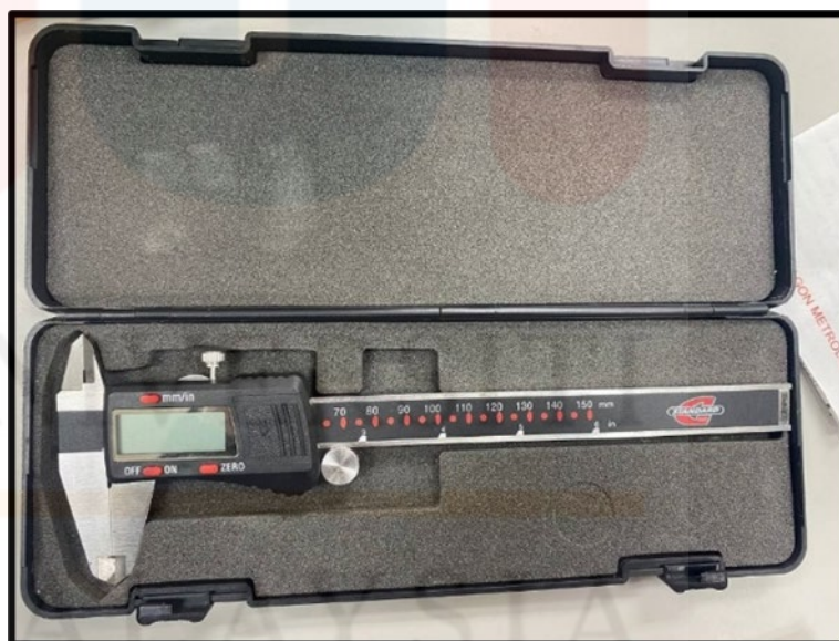
Figure 3.4 Digital vernier calliper
