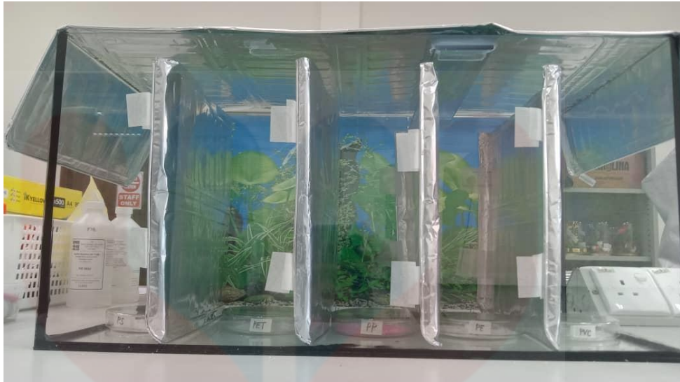
Figure 3.4: The aquarium was partitioned into five compartments, each containing a different type of plastic placed in Petri dishes.
