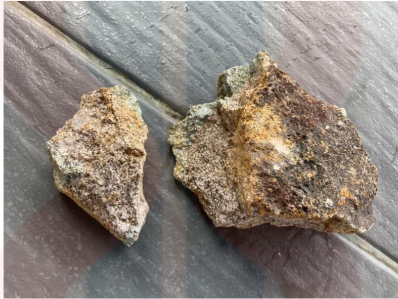
Figure 4.17: Hand specimen (macroscopic) of alkali-feldspar granite labelled as OC1
