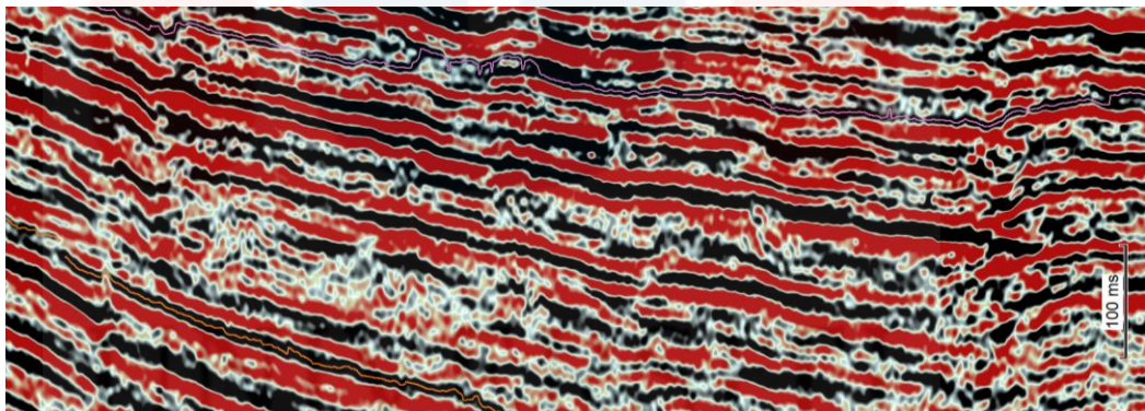
Figure 5.12: Divergent reflection on Line C21 Residual absorption
