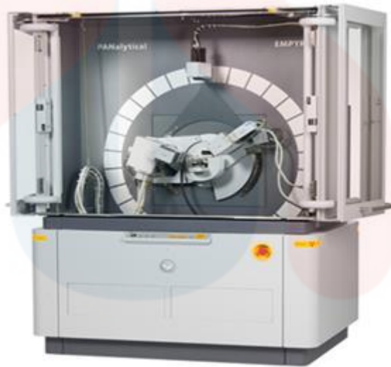
Figure 3.2: X-ray Powder Diffraction instrument.
