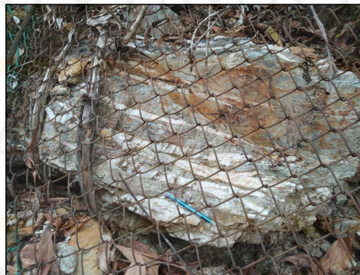
Figure 4.19 A boulder that was separated from the rock mass due to physical weathering.
