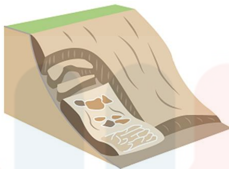
Figure 2.43 : Translational slides (British Geological Survey)
