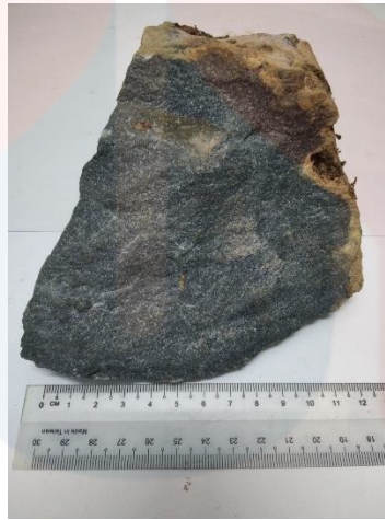
Figure 4.21: Hand specimen of hornfels rock at JL12
