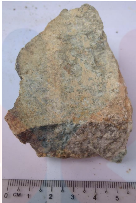
Figure 4.17: Hand specimen of granite at JL9
