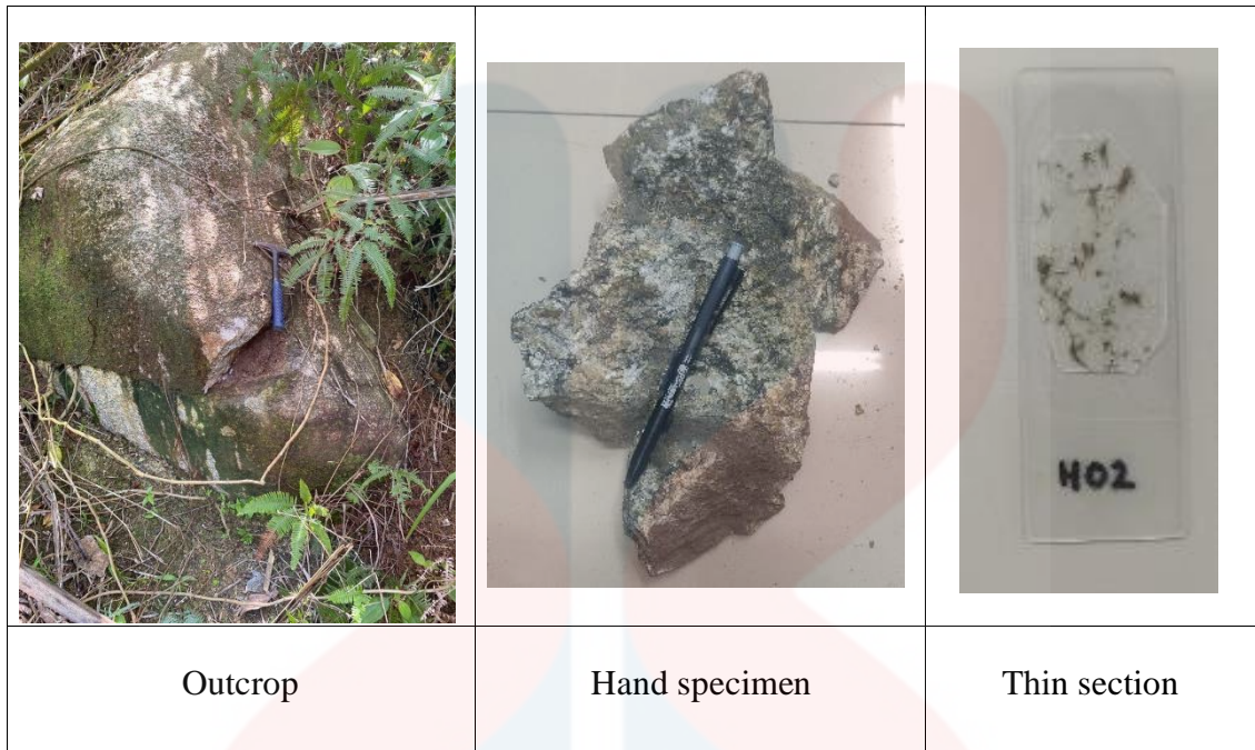
Figure 4.17: Outcrop, Hand specimen and Thin section for Granite Sample 2
