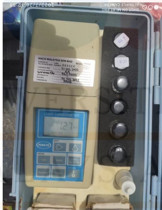
Figure 3.2: Water sample wells around Kampung Panglima Baru utilised 2100P portable turbidity metre to record the turbidity.
