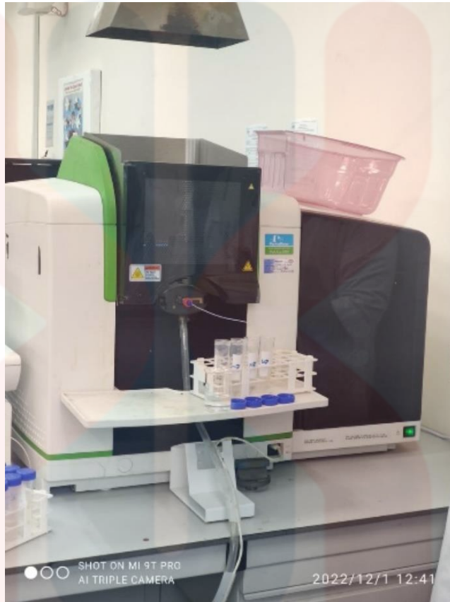
Figure 3.4: The AAS PinAAcle 900F instrument used to analyse major cation concentration
