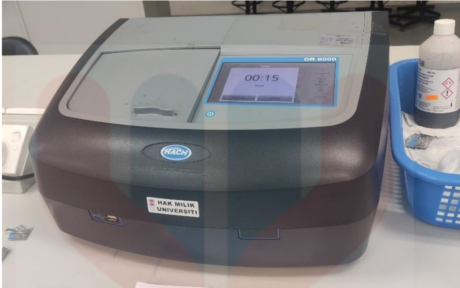
Figure 3.6: The Spectrophotometer DR6000 instrument used to analyse major anion concentration
