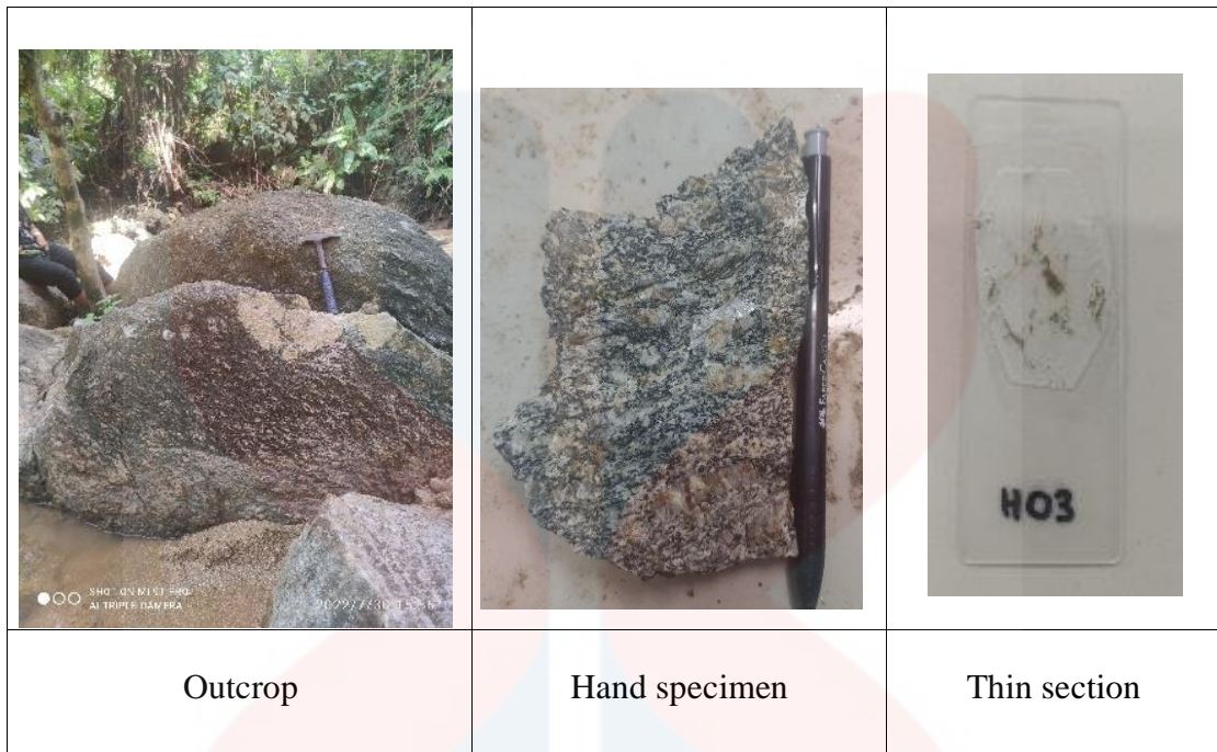
Figure 4.19: Outcrop, Hand specimen and Thin section for Granite Sample 3
