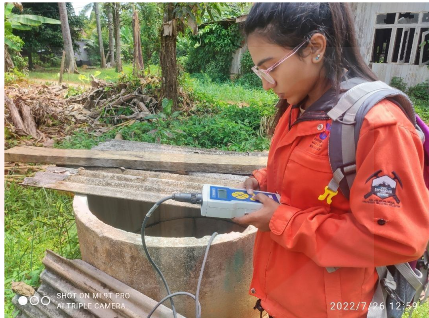
Figure 3.3: Water sample wells around Kampung Panglima Baru utilised YSI 556 MPS Multi-parameter instrument to record in-situ parameters.
