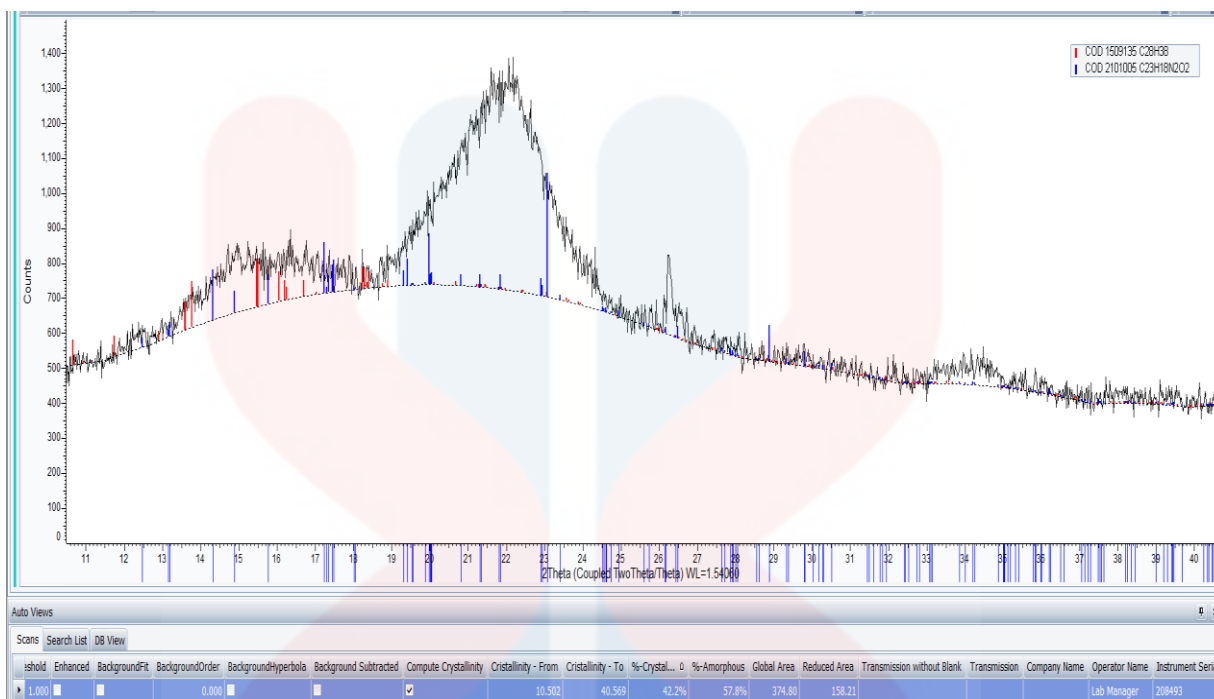
Figure 13: XRD analysis for rubberwood sawdust for 10% Urea-Formaldehyde
