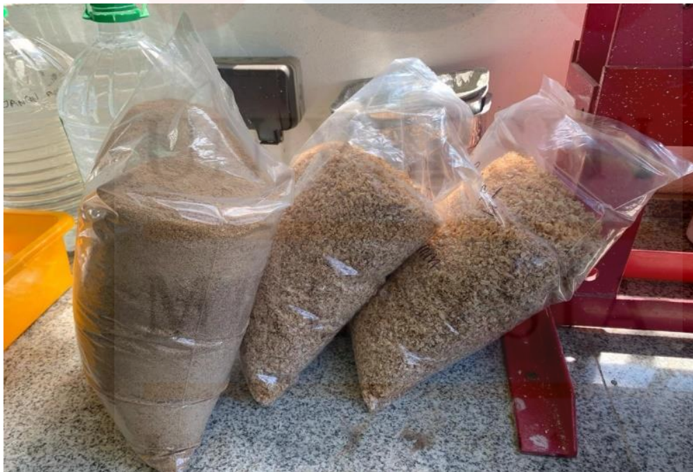
Figure C(b): Rubber wood dust that has been sieved and separated according to size.
