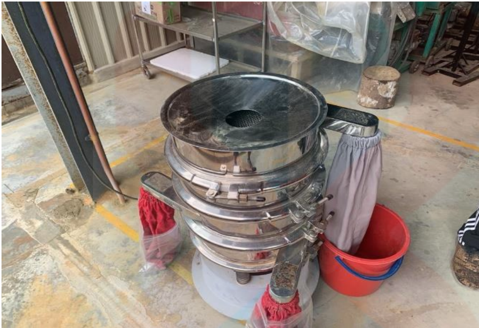
Figure C(a): Sieve machine for sifting thick rubber wood dust.
