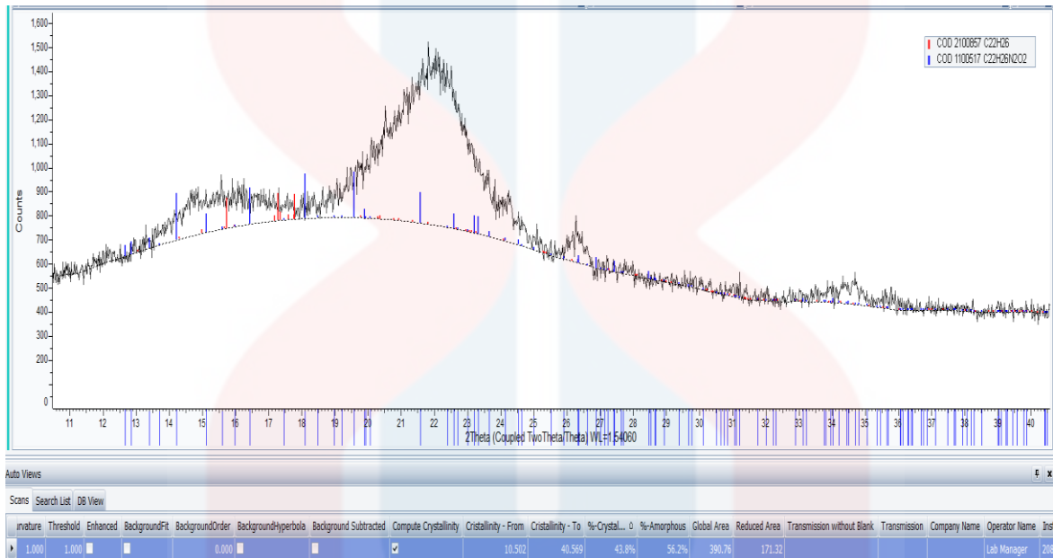
Figure 11: XRD analysis for rubberwood sawdust for 30% Urea-Formaldehyde
