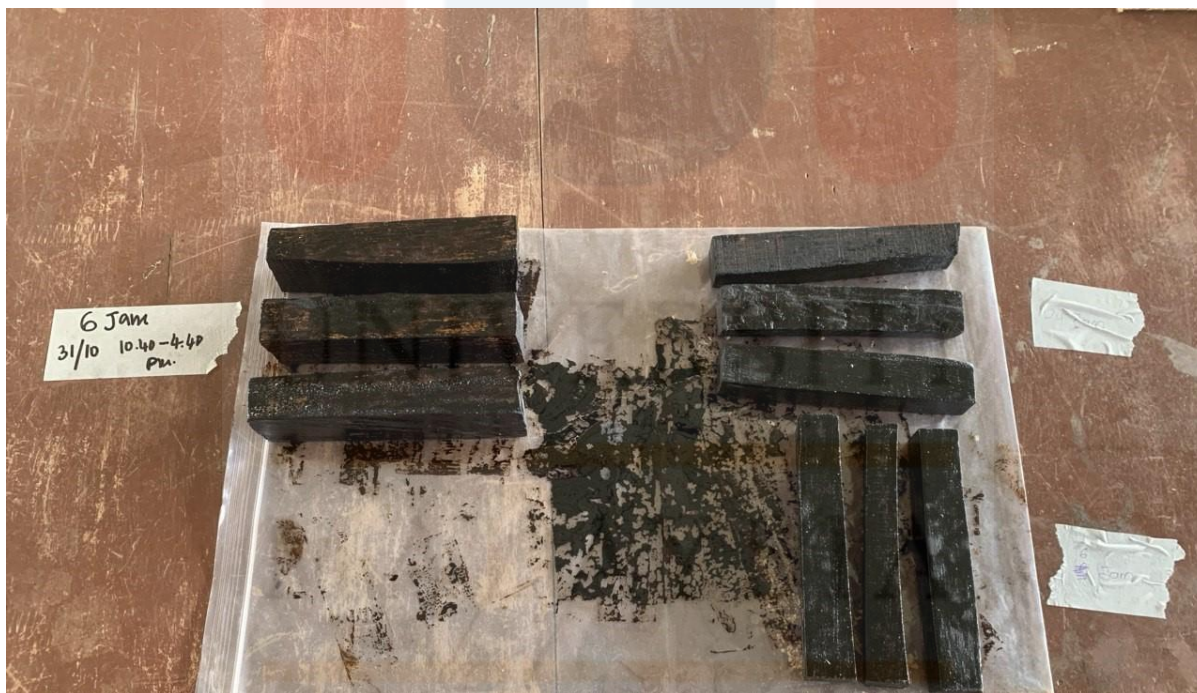
Figure B.2: Acacia wood dried room temperature before oven dry.
