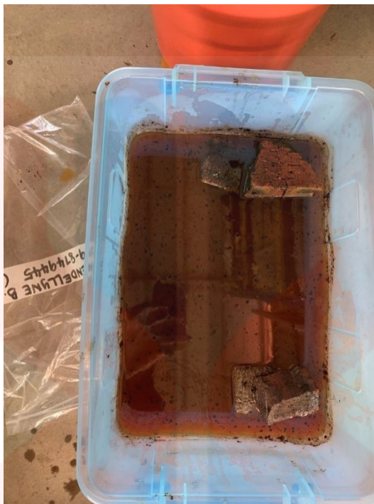
Figure B.1: Acacia wood soaked into wood vinegar and silica extracted rice husk ash.
