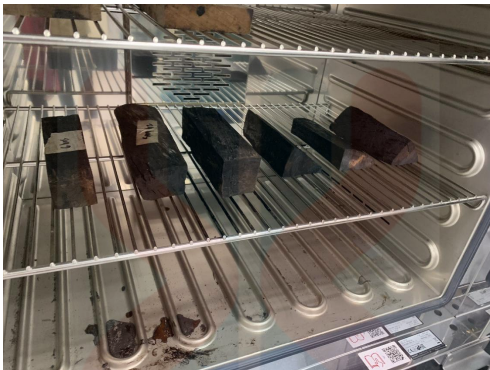
Figure B.3: Acacia wood has been thermal after soaked in preservatives.
