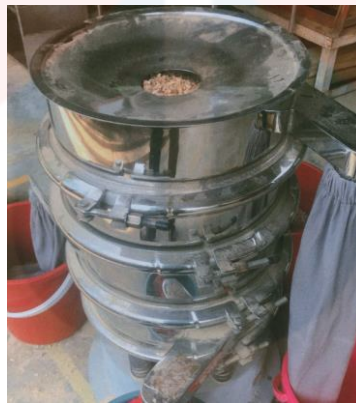
Figure 31: Separating the rubber wood dust which is divided into four, i.e. Free, 100mm, 150mm, 750mm into a sieved machine
