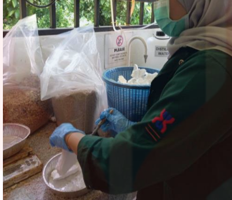
Figure 33: The polystyrene was melted using acetone.
