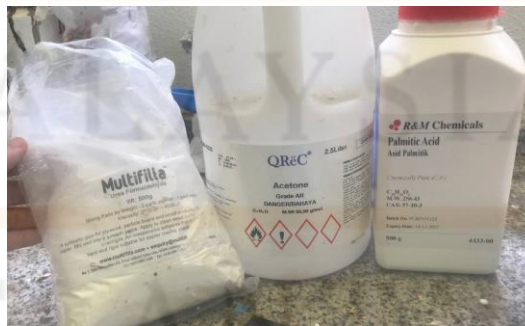
Figure 32: Materials were mixed with polystyrene and wood dust along with UF and palmitic acid. Acetone was used to dissolve the polystyrene.
