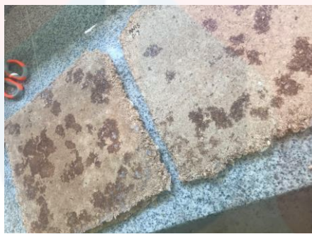
Figure 37: The shape of the particleboard was released from the hot press.
