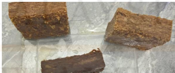
Figure 23: Sample 24 hour soaked in the water for sample DT0.6 \text{g/cm}^3 , DT0.7 \text{g/cm}^3 , and DT0.8 \text{g/cm}^3 .
