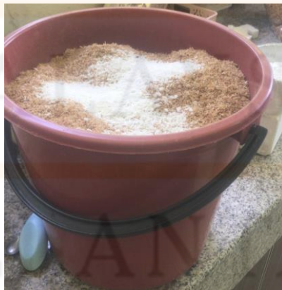
Figure 35: The UF and PA were mixed into rubber wood dust that had been mixed with PS.
