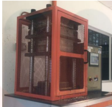
Figure 36: The hot press machine was used to press wood dust mixed with PS, UF, and PCM to make particleboard.
