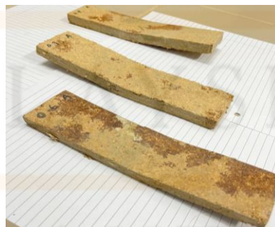
Figure 26: Wood composite for sample DT DT0.6 g/cm^3 , DT0.7 g/cm^3 , and DT0.8 g/cm^3 after testing
