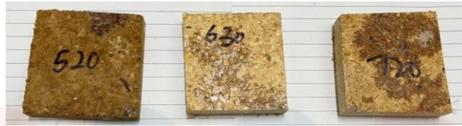
Figure 20: Sample before soaked in the water for sample DT0.6 \text{g/cm}^3 , DT0.7 \text{g/cm}^3 , and DT0.8 \text{g/cm}^3 .
