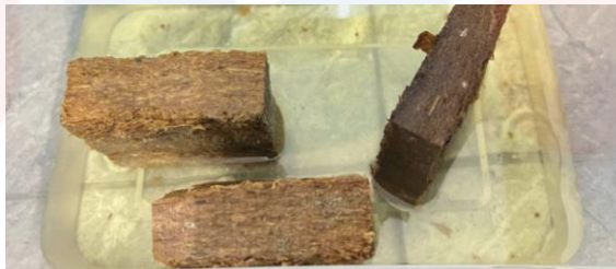
Figure 22: Sample 2 hour soaked in the water for sample DT0.6 \text{g/cm}^3 , DT0.7 \text{g/cm}^3 , and DT0.8 \text{g/cm}^3 .
