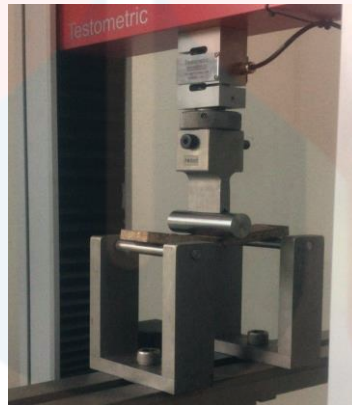
Figure 25: Bending machine process bending particleboard for DT0.6 g/cm^3 , DT0.7 g/cm^3 , and DT0.8 g/cm^3
