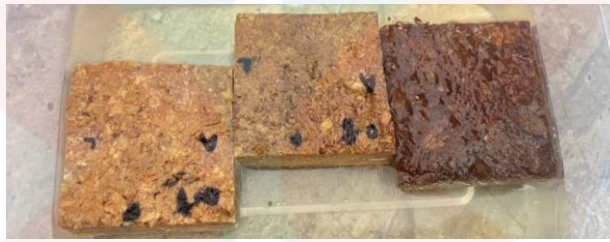
Figure 21: Sample 1 hour soaked in the water for sample DT0.6 \text{g/cm}^3 , DT0.7 \text{g/cm}^3 , and DT0.8 \text{g/cm}^3 .
