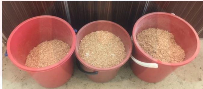
Figure 34: Rubber wood dust that had been separated according to the specified density.
