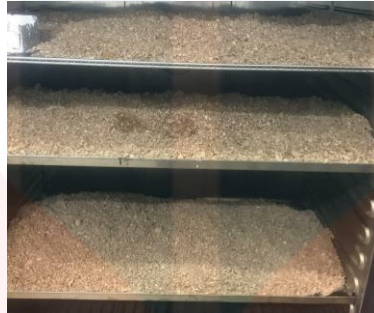
Figure 30: Dried the wood dust for 24 hours in oven.
